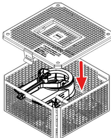
4. Before sterilizing, pack the RESIGHT metal tray with the components into a suitable container with a sterile barrier (e.g. a sealed bag). The sterilization container and the filter must comply with ISO 11607-1:2006.
