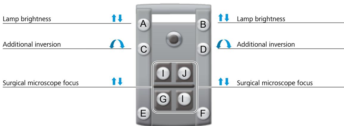
Figure 20: Button assignments with RESIGHT 700 out of the beam path
