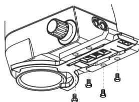
5. Push the mounting aid away from the main camera lens of the surgical microscope so that the cutouts on the mounting aid line up with those on the adapter plate.
