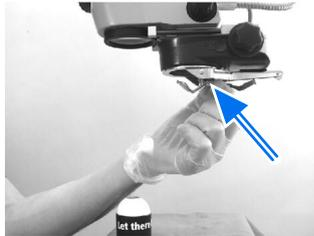
2. Apply counterpressure to the joint with the back of your thumb to detach the lens support mechanism from the magnetic lock.
