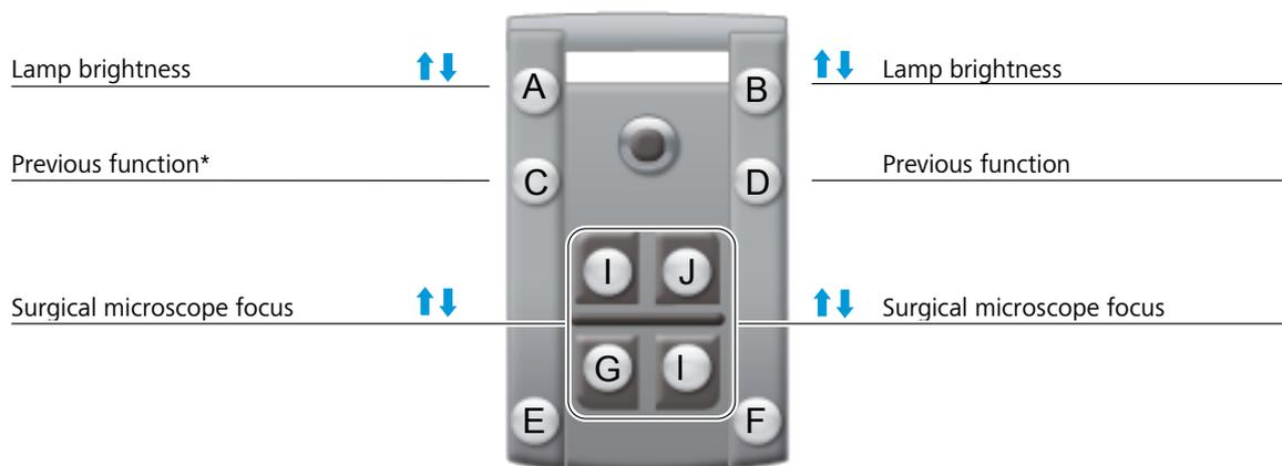
Figure 18: Button assignments with RESIGHT 700 out of the beam path
