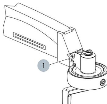
Figure 25: Adjusting the downward travel limit, example with S88 / OPMI Lumera T
