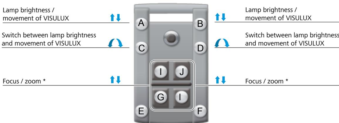
Figure 12: Button assignments with VISULUX connected
