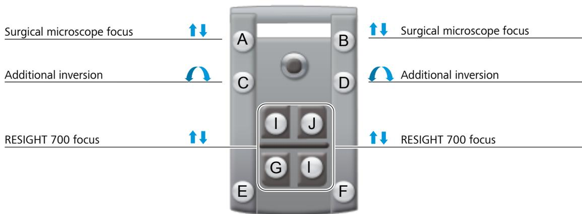
Figure 19: Button assignments with RESIGHT 700 in the beam path
