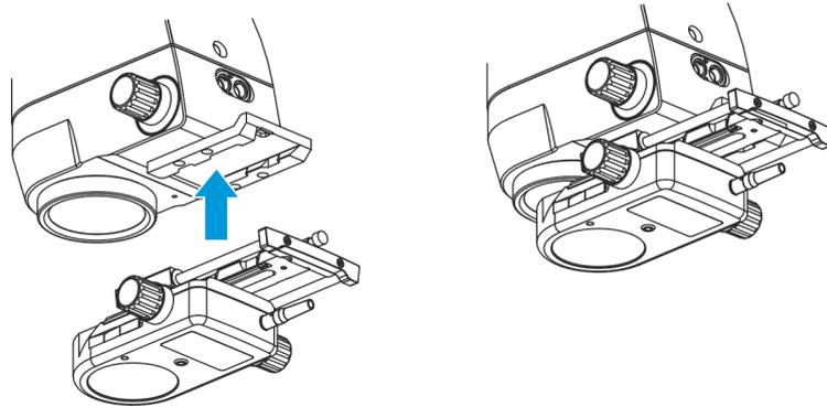
2. Push the focusing unit on the adapter plate in the direction of the objective lens of the surgical microscope up to the end stop until the focusing unit audibly snaps into place.
