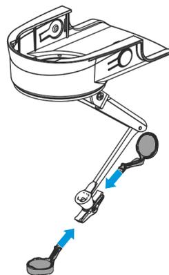
2. Unfold the sterile lens support and slide it onto the focusing unit from the front until it audibly clicks into place.
