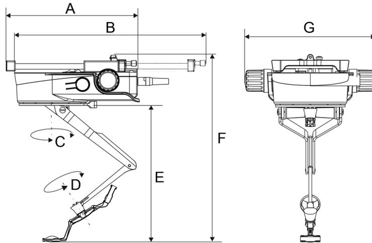
Figure 26: Dimensions and swiveling ranges
