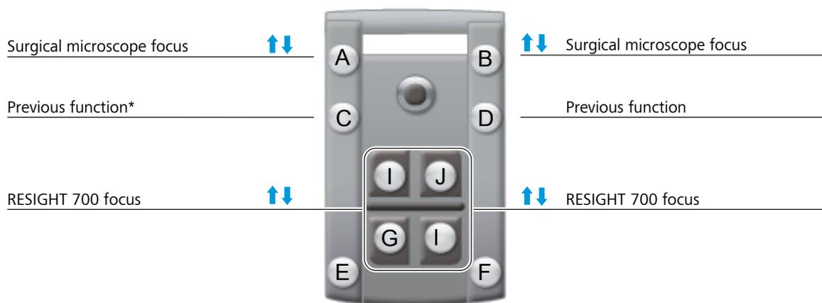
Figure 17: Button assignment with RESIGHT 700 in the beam path
