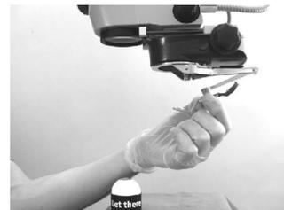
3. Slowly pull down the lens support mechanism until it has folded out completely.
