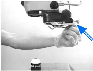
2. Slowly pull down the lens support mechanism at the hinge until it has folded out completely. Make sure not to touch the non-sterile RESIGHT fundus viewing system in this process.
