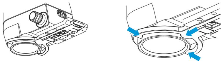
4. Screw the adapter plate in place under the surgical microscope by firmly tightening the four accompanying screws clockwise. Ensure that the three alignment points in the mounting aid are touching the camera lens of the surgical microscope.
