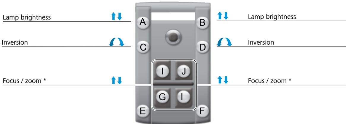
Figure 13: Button assignments with Invertertube E connected
