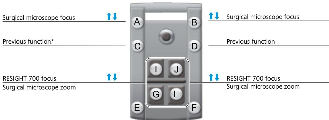
Figure 15: Button assignment with RESIGHT 700 in the beam path
