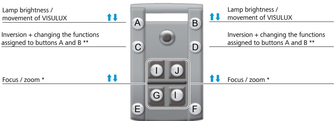
Figure 14: Button assignments with Invertertube E and VISULUX connected
