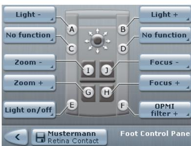
Tip: Test the button assignments and functions on the 14-function foot control panel before each use when the patient is not present.
