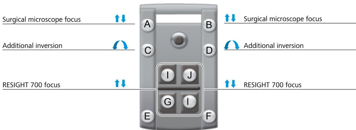
Figure 21: Button assignments with RESIGHT 700 in the beam path
