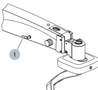
Figure 24: Adjusting the downward travel limit on the OPMI Lumera i
