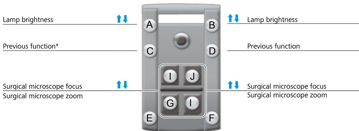
Figure 16: Button assignments with RESIGHT 700 out of the beam path
