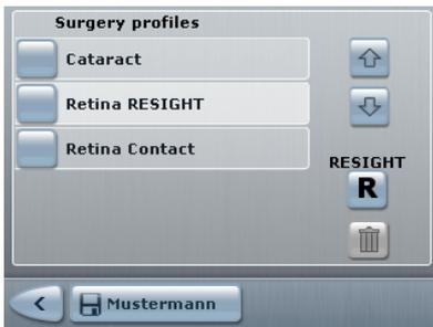
If the RESIGHT function has been assigned to a surgery profile (surgery profile is identified with an "R"), you can assign the focus control of the surgical microscope (focus + / focus -) and of the RESIGHT fundus viewing system (RESIGHT focus + / RESIGHT focus -) to any button of the foot control panel.
