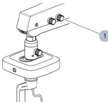
Figure 23: Adjusting the downward travel limit on the OPMI Lumera 300
