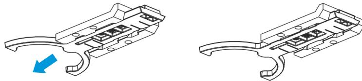
3. Adjust the adapter plate with the help of the mounting aid on the surgical microscope. The three alignment points in the mounting aid must make contact with the camera lens of the surgical microscope.
