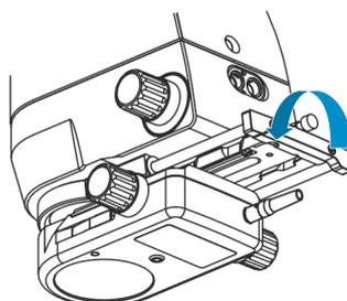
3. Press and hold down the unlocking button and pull the focusing unit backwards from the adapter plate.
