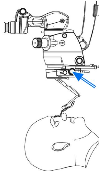
5. The surgical microscope no longer needs to be vertically moved for focusing. When working on the anterior segment, you can therefore move the RESIGHT fundus viewing system out of the beam path without causing blurring of the image.
