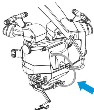
2. Hold the focusing unit with one hand and loosen the locking screw. Turn it counterclockwise.
