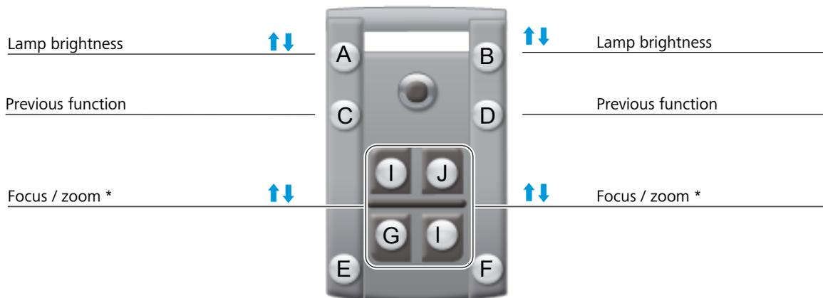
Figure 11: Button assignments if Invertertube E, RESIGHT and VISULUX are not connected
