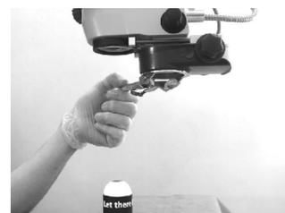
3. Slowly pull down the lens support mechanism at the hinge until it has folded out completely.
