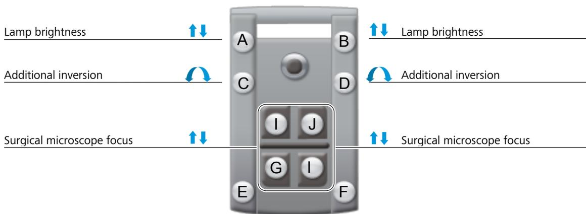
Figure 22: Button assignments with RESIGHT 700 out of the beam path
