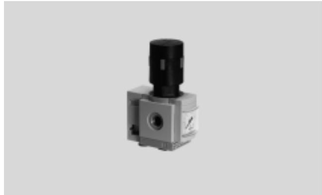
The pressure regulator is suitable for manifold assemblies with through air supply, for configuring a regulator manifold with separate, independent pressure regulation ranges. Pressure output is to the front or rear.
