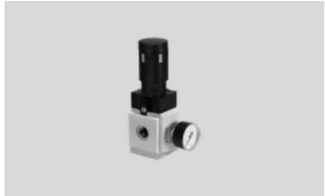
The precision pressure regulator is suitable for sensitive applications with a required hysteresis of 0.02 bar. The output pressure p2 can be set within the pressure regulation range either manually using the rotary knob or pneumatically via a pilot pressure p12
