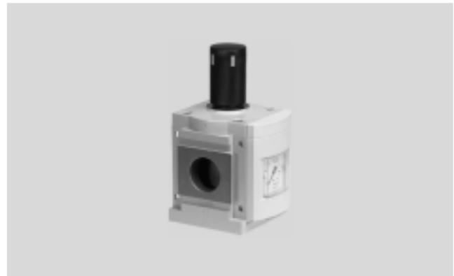
The pressure regulator maintains an essentially constant output pressure p2 independent of pressure fluctuations in the system and air consumption. The output pressure p2 can be set within the pressure regulation range either manually using the rotary knob, pneumatically via a pilot
