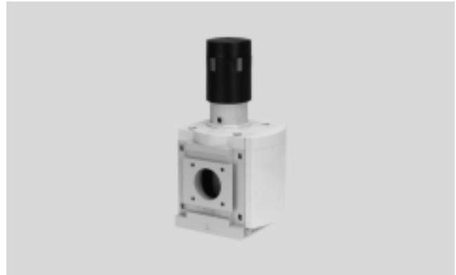
The pressure regulator maintains an essentially constant output pressure p2 independent of pressure fluctuations in the system and air consumption. The output pressure p2 can be set within the pressure regulation range either manually using the rotary
