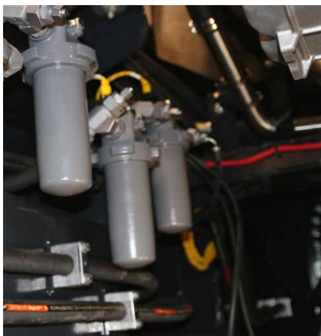
Hydraulic filter system.
