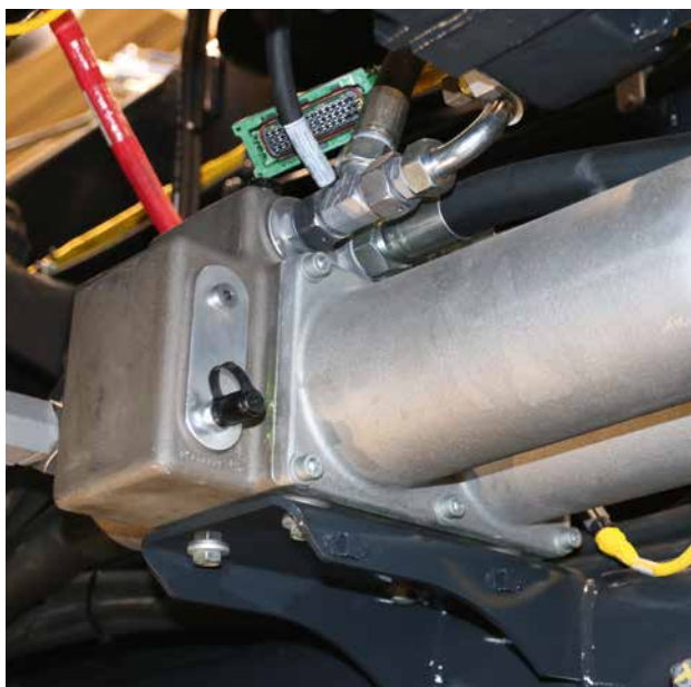
Electronic monitoring of hydraulic return filter.
