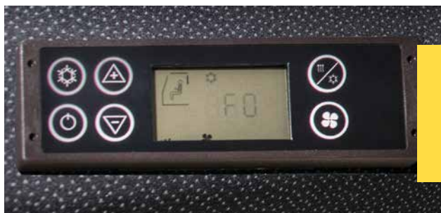
Automatic heating and air-conditioning unit control panel.
