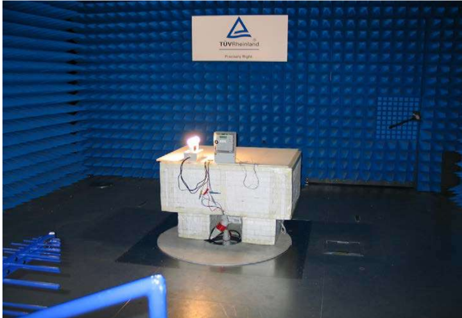
Photograph of the radiated emission test:
