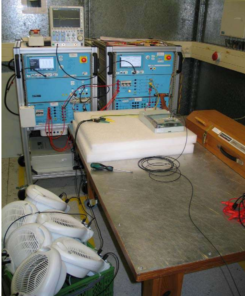
Photograph of the damped oscillatory waves immunity test:
