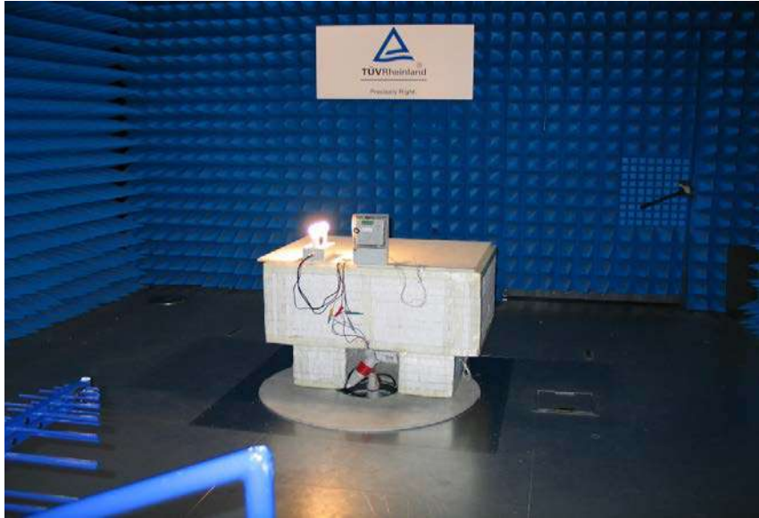
Photograph of the conducted emission test:
