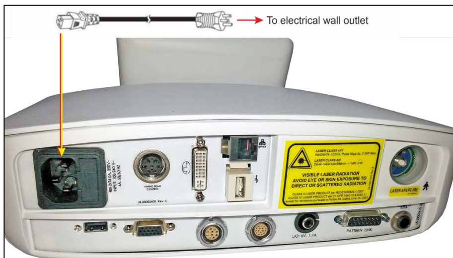
Figure 4-6: Connecting the Main Power Cable
