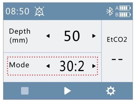
Figure 31 Pressing mode setting
