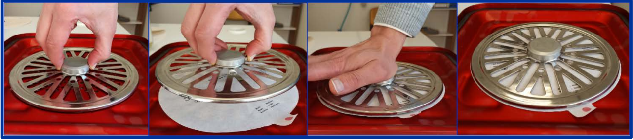
Figure 9. Removing and attaching the filter retainer and changing the filter.
