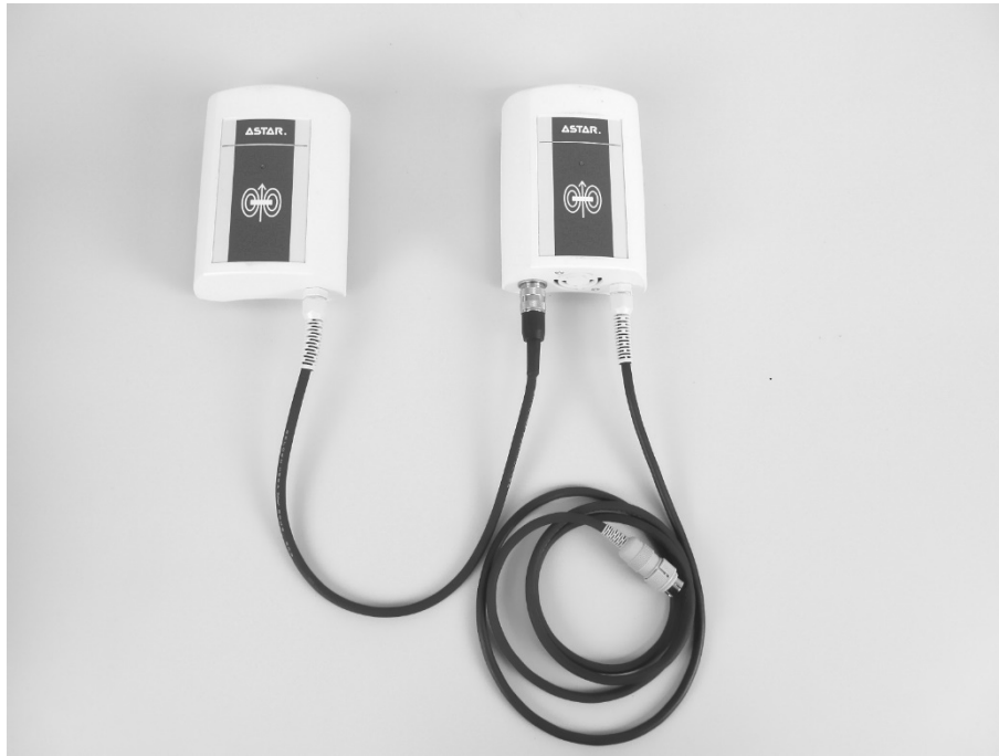
Figure 3.4. Connected magnetic field applicators – CPE type
