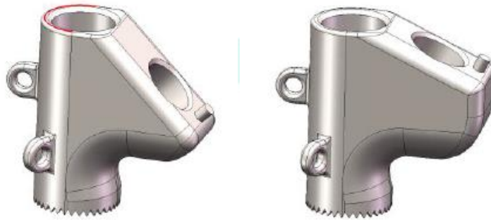
Fig. 16. AGILON® METAPHYSEAL COMPONENT TRAUMA (135° LEFT, 155° RIGHT)
