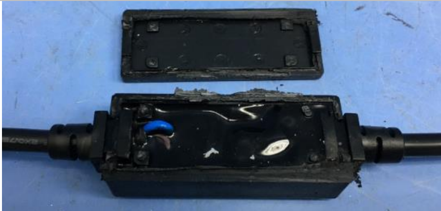
Interna View of Rectifier with Potting Compound
