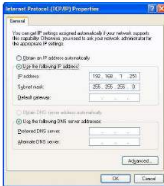
Figure 254: Static IP address settings for the Slave PC
