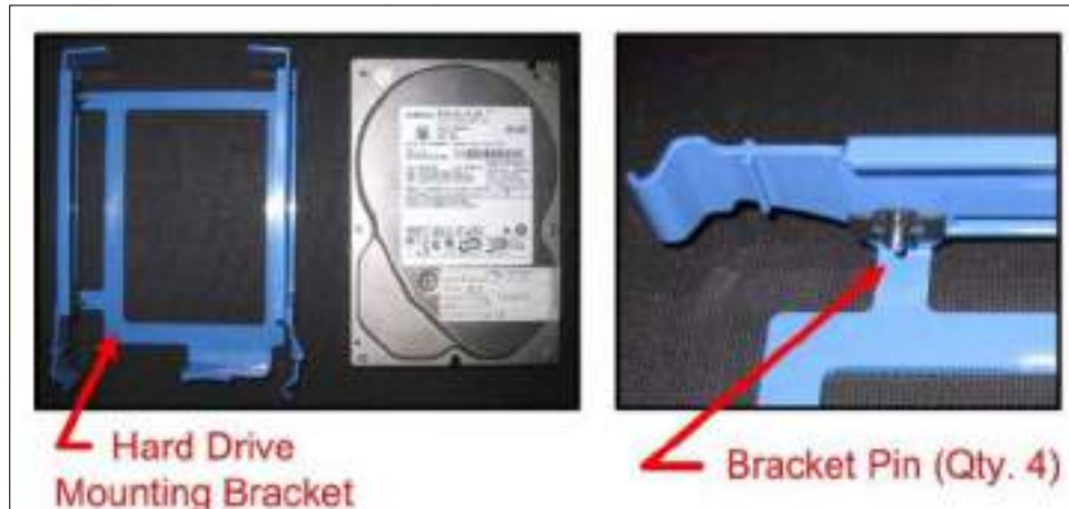
Figure 153: Removing Hard Drive from Mounting Bracket
