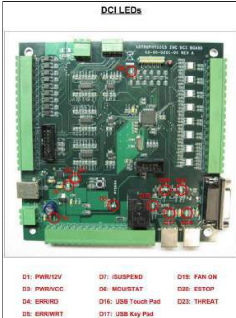
Figure 175: DCI Board LEDs
