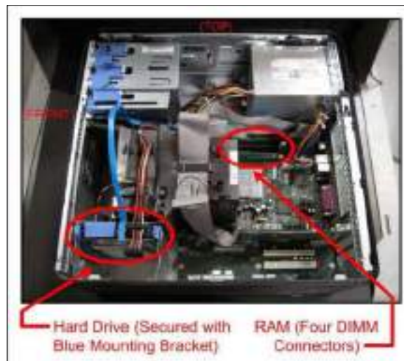
Figure 149: PC Internal Layout
