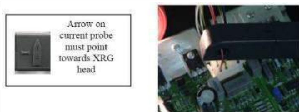
Figure 101: Current Probe Used to Observe mA Drive Signal
