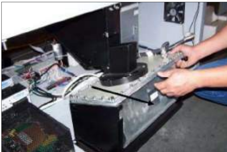
Figure 206: Removing the Generator
