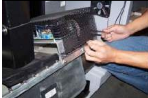
Figure 197: Removing Generator Control Board Cover
