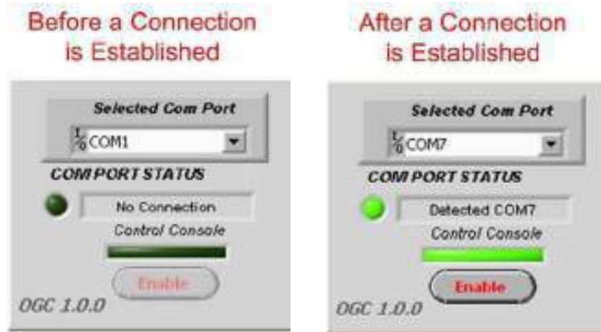
Figure 235: Connecting to the Proper COM Port with the COM Selector
