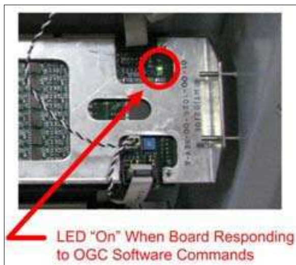
Figure 239: LED Component "D-1" on the LXDA 2.0 Low-Energy Side
