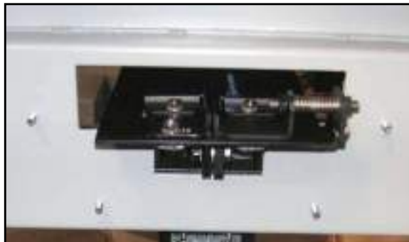
Figure 76: Collimator Bars and Gap Adjustment Screw
