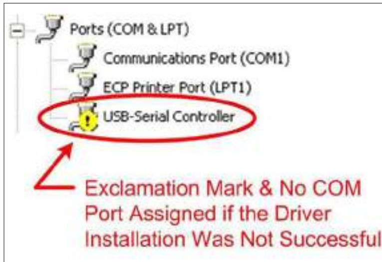
Figure 247: Unsuccessful Installation and Assignment of COM Port to USB-Serial Adapter Cable
