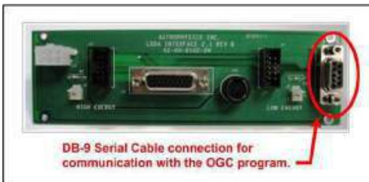
Figure 225: LXDA Interface Board, 2.1, Rev B
