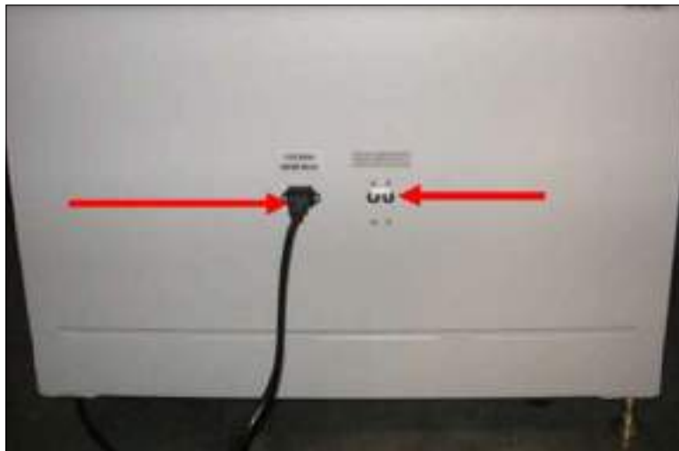
Figure 16: AC Power Cord and Main Circuit Breaker Switch
