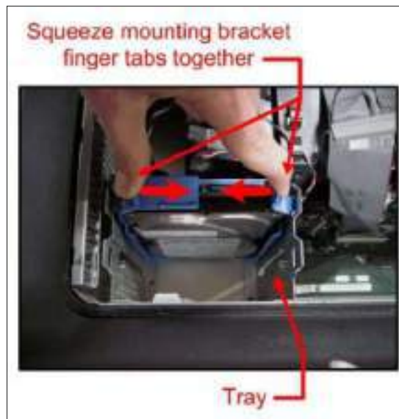
Figure 152: Removing Hard Drive from Tray Slot
