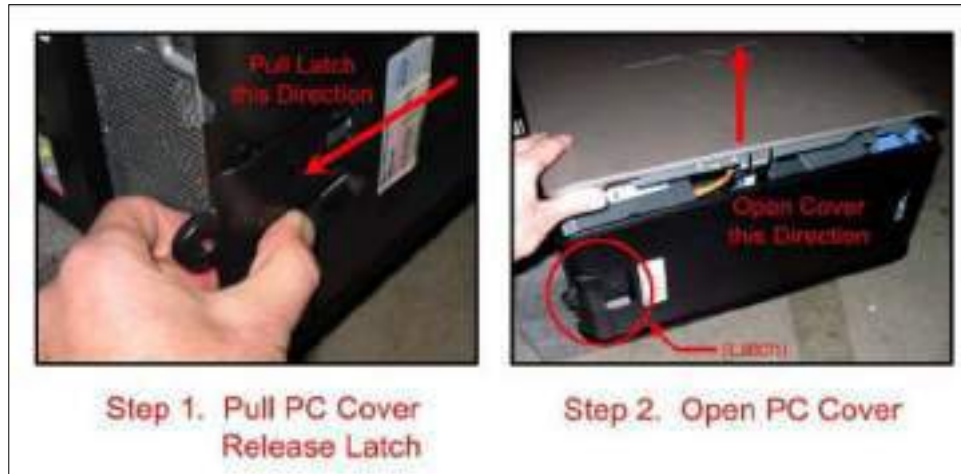
Figure 148: Opening the PC Cover
