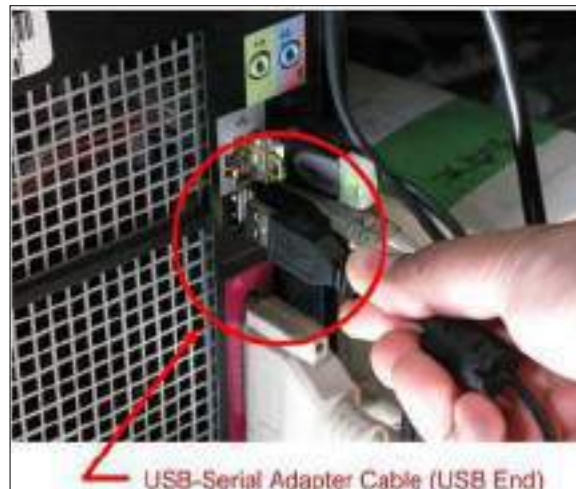
Figure 228: USB-Serial Adapter Cable to PC Connection
