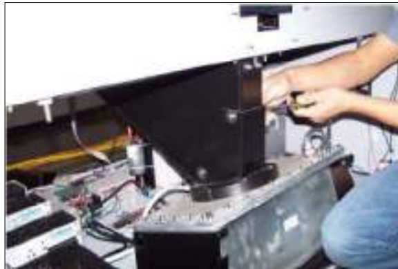
Figure 203: Removing Funnel Cover Mounting Screws
