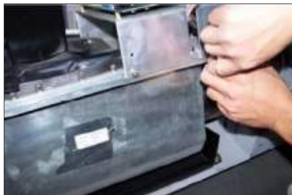
Figure 201: Undoing Control Board Mounting Screws
