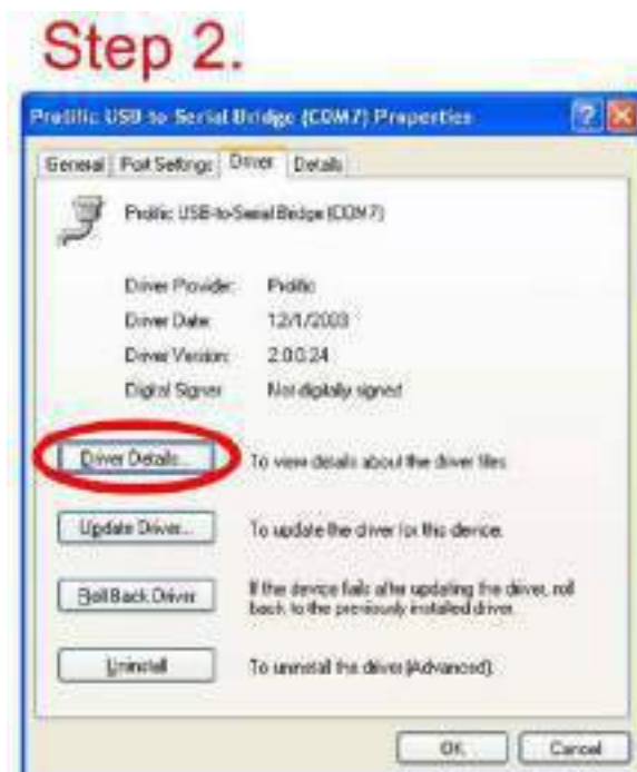
Figure 249: Step 2 Confirming File Name of USB-Serial Adapter Cable Driver
