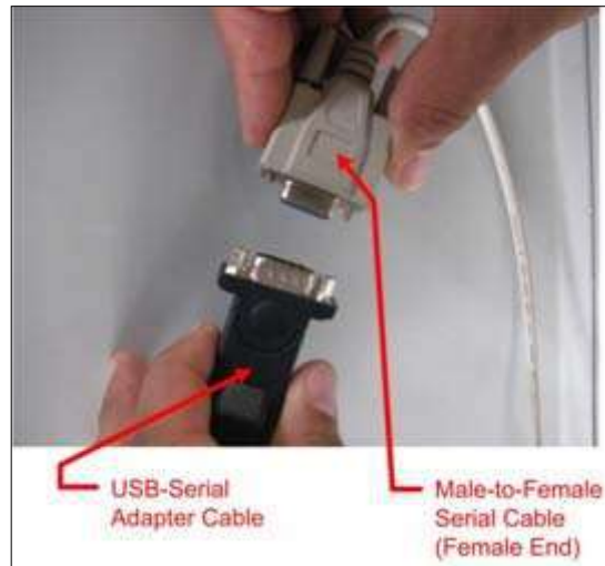
Figure 230: USB-Serial Adapter Cable to Serial Cable Connection
