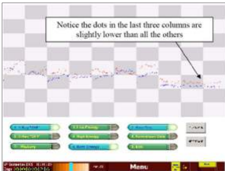
Figure 216: Diode Plot Showing Misalignment
