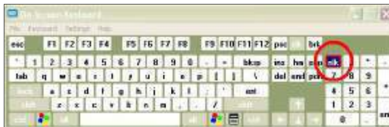
Figure 160: Windows XP On-Screen Keyboard “nlk” (Num Lock) Button
