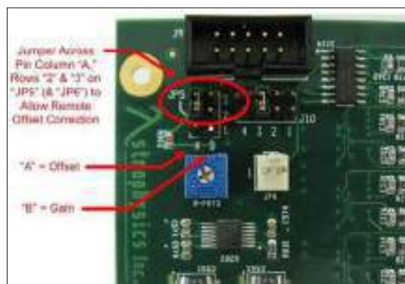
Figure 223: Remote Offset Correction Selected on High Energy Side (“JP5”)
