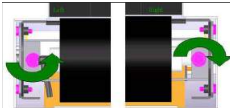
Figure 70: Left Bolt Counterclockwise, Right Bolt Clockwise
