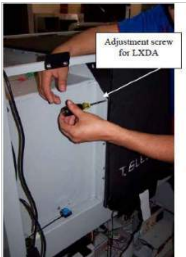
Figure 217: LXDA Adjustment Screw
