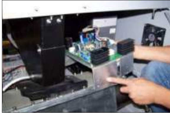
Figure 202: Removing the Control Board
