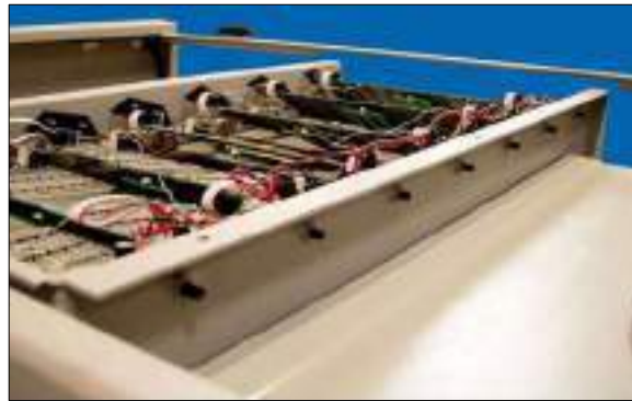
Figure 79: Collimation screws for individual LXDA Boards.
