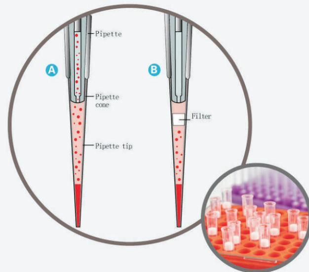
Experiment prove tips with filter will work better under enviroment condition which with particle.
