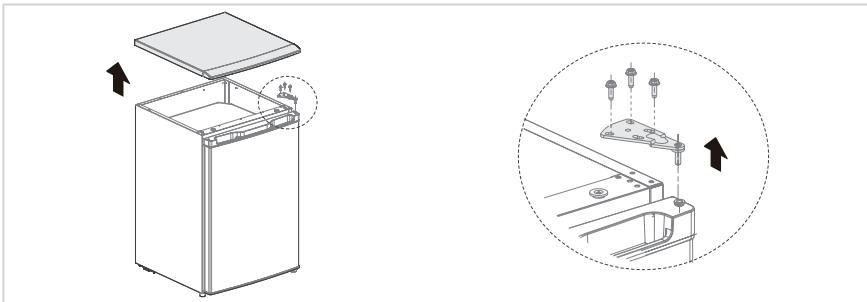
3. Dismantle the door and the bottom hinge assembly and adjustable foot, then assemble the bottom hinge assembly and adjustable foot on other side.
