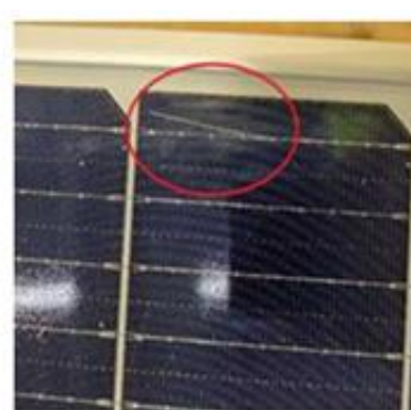
fig.3 Damaged bus bar
