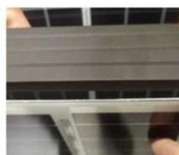
fig.6 No silicone or glue connecting the frame to the inner parts
