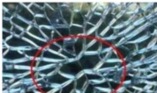
fig.1 Spontaneous cracking - point in a "butterfly" shape
