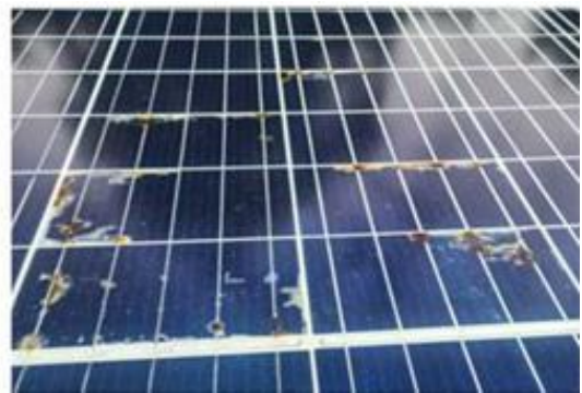
fig.2 Spot burns visible
