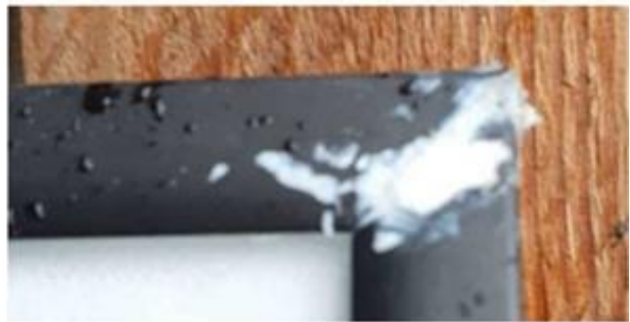
fig.5 Silicone residues from the production process
