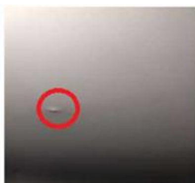
fig. 2 Foreign body - laminate side
