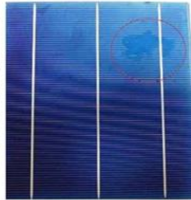
fig.3 Defect under glass
