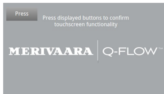
Picture 41. The diagnostic test of the touchscreen.
