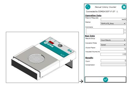
On the panel, you can see on the top whether a DOT instrument has been found connected to the SphereFlash<sup>®</sup> application.
