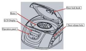
Figure 5.1 Front view of the centrifuge
