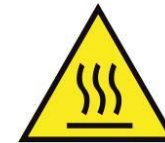
CAUTION HOT SURFACE Caution hot surface
