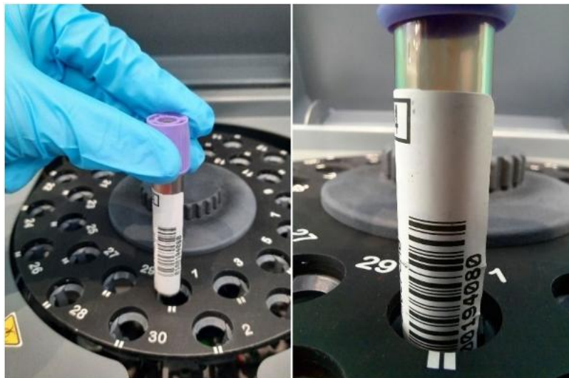
Figure 24 Correct insertion of the test tube
