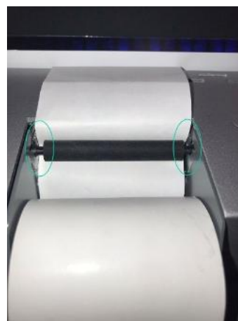
Figure 20 - Printer paper replacement: correct position
