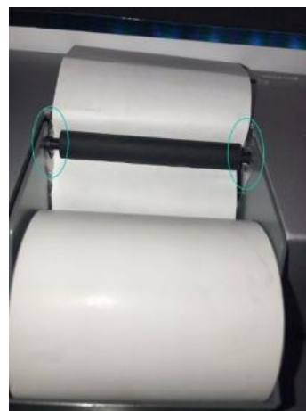
Figure 18 - Printer paper replacement: roll off axis
