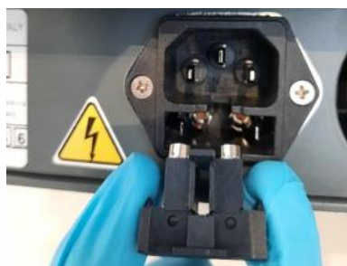
Figure 17 – Replacement of the fuses: repositioning box
