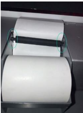
Figure 19 - printer paper replacement: pin off axis
