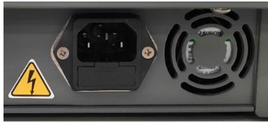
Figure 14 – Replacement of the fuses: fuses box
