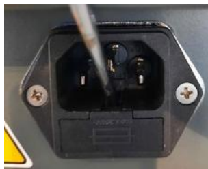
Figure 15 – Replacement of the fuses: extraction box
