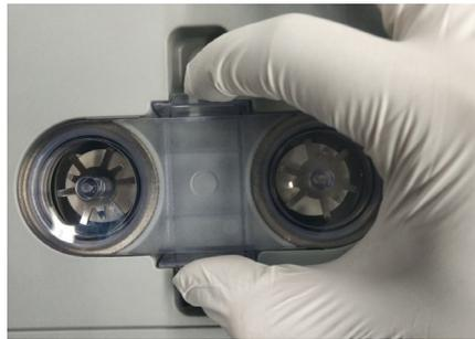
**FIGURE 12-23** Install the Check Valve Cover
