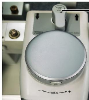
Locking mechanism handle in the unlocked position
