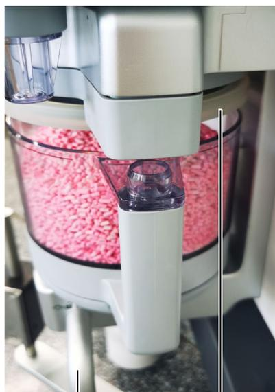
**FIGURE 12-32** Canister Unlocking
