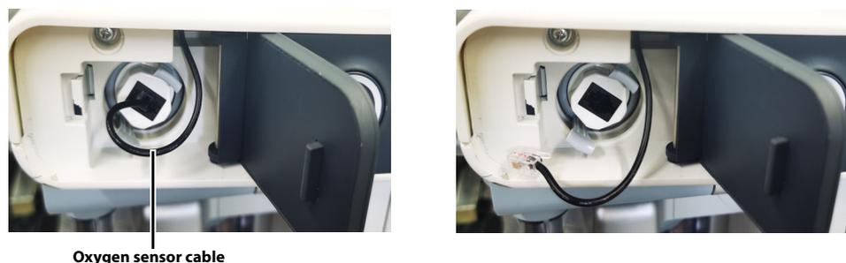
**FIGURE 12-5** Pull Out the O<sub>2</sub> Sensor Cable
