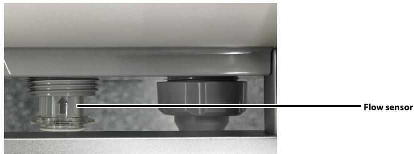
**FIGURE 12-26** Install the Flow Sensor
