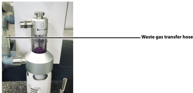
**FIGURE 12-43** Remove the Waste Gas Transfer Hose
