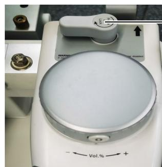
Locking mechanism handle in the locked position
