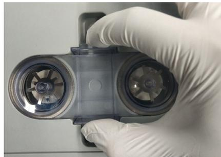
**FIGURE 12-18** Remove the Check Valve Cover
