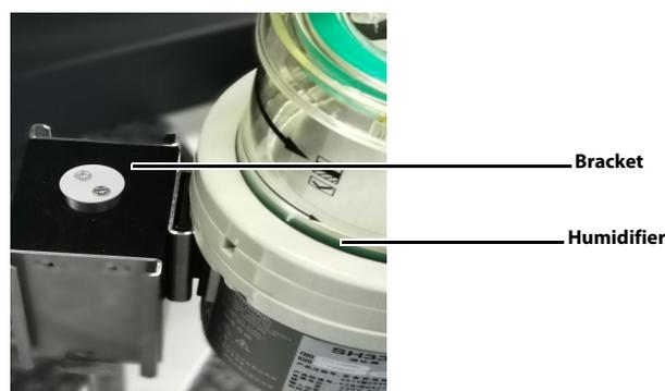
**FIGURE 3-9** Install the Humidifier
