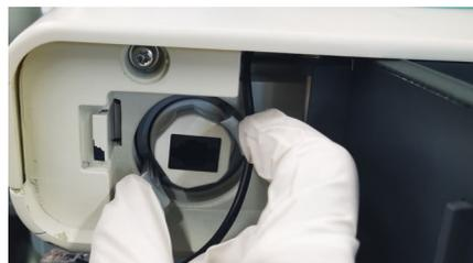
**FIGURE 12-36** Install the O<sub>2</sub> Sensor Support
