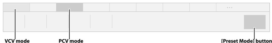
**FIGURE 6-6** Press the **[Preset Mode]** Key to Set PCV as the Ventilation Mode upon Exit from the ACGO Mode
