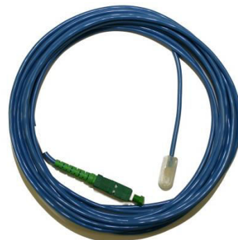
Temperature sensor for surface (axilla / armpit) temperature measurement
