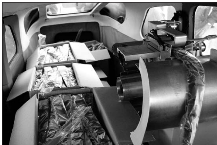
FIGURE 2: The dropping device of the SURVIS-system together with baits wrapped in flexible foil tube (A) and the sensor for recording of individual bait release (B).
