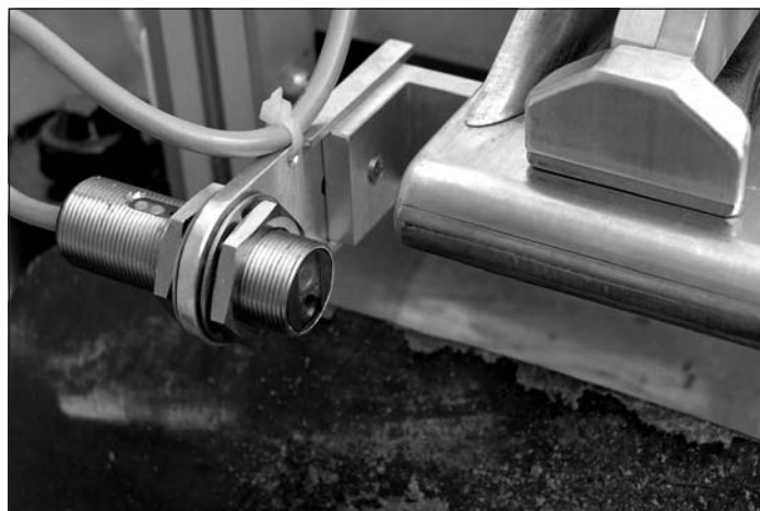
FIGURE 2: The dropping device of the SURVIS-system together with baits wrapped in flexible foil tube (A) and the sensor for recording of individual bait release (B).
