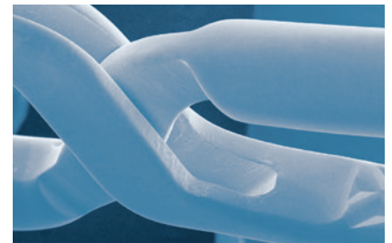
REM image unique box lock of a YASARGIL Clip from Aesculap; the flat design with a broad contact surface enables smooth opening and closing as well as stability.
