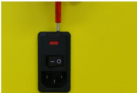
The two main fuses are accessible from outside and positioned in the power input module behind a protective cover.
