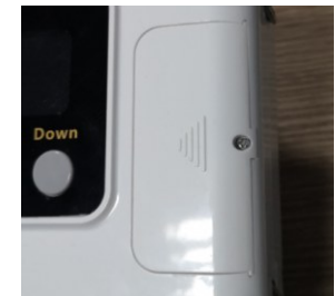
Step 10: Close the battery house cover and screw in the screws.
