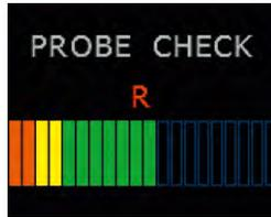
Feedback on the placement of the probe
