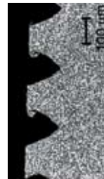
Deformed taper structure after 61 months in vivo
