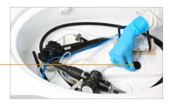
N.B. Place the endoscope inside the basin, paying attention to locate it below the spray arm (rotating arm located on the cover). In addition, ensure that
