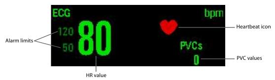
PVCs values is shown only when arrhythmia analysis is switched on. When external paddles or multifunctional electrode pads are used for ECG monitoring, the PVCs values is shown as "---".
