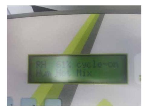
\* If there need to stop the automatic cycle (not recommended), press autocycle button on the panel continuously for 4 seconds.
