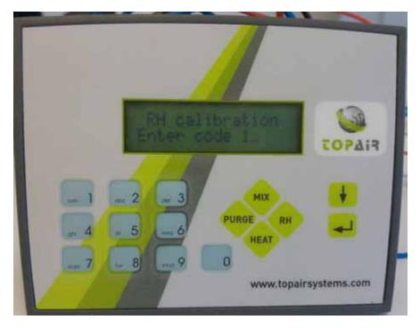
2. Press the calibration code '1' on the keypad and press the Enter arrow key.
