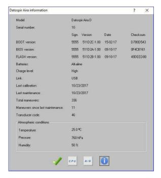
CPU test: checks the proper functioning of the spirometers's electronics.
