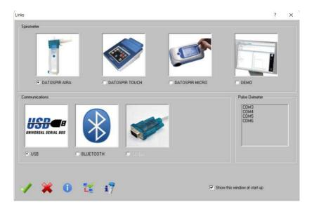
This dialog is used to select the spirometer used to make the tests and the communications link used to transfer data to the PC.
