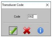
This code will be applied by the equipment, and will always appear in the title line of the results summary window. It is also possible to modify this code through the Transducer Code option in the Setup menu. This code must be entered only once while the code of the disposable transducers remains the same. If the lot is not yet added to the program, the next window will appear to enter the K values:
