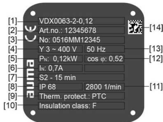
Figure 3: Motor name plate (example)
