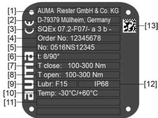
Figure 2: Actuator name plate (example)
