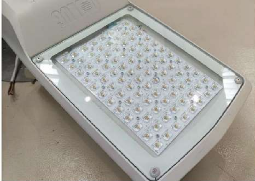
Photograph No. 3 Detail of light emitter surface after IK 09 test (no breakages on glass)
