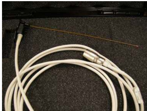
Figure 13-151. Needle Tip Sensor and Cable Close-up
