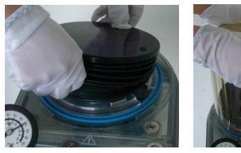
Figure 3-5 Folding bag and bellows housing installation view
