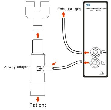
Figure 6-1 Sidestream analyzer connection view
