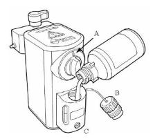
Figure 3-17 Adding anesthetic view
