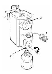
Figure 3-18 Discharging anesthetic view
