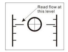
Figure 2-7 Flowmeter float indication
