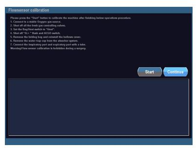
Figure 5-5 Flow sensor calibration screen
