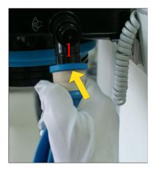
Figure 3-15 Manual breathing bag installation view
