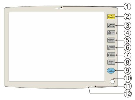
Figure 2-12 Membrane button view
