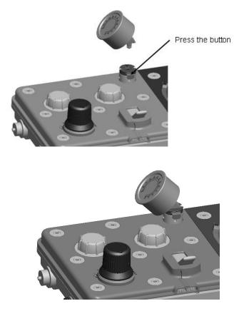
Figure 3-6 Micro manometer installation view
