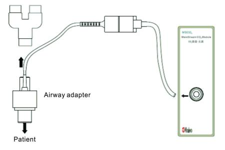
Figure 6-2 Mainstream analyzer connection view
