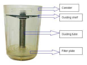
Figure 3-8 Canister view
