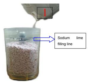
Figure 3-9 Absorbent filling view
