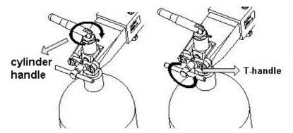
Figure 3-2 Gas cylinder connection view I
