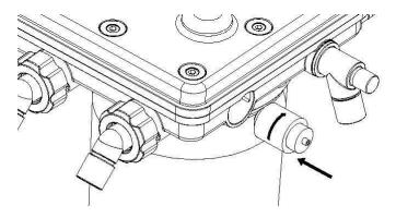
Figure 3-7 Oxygen sensor installation view
