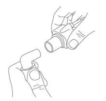
Figure 6-6 IRMA airway adapter connection view II
