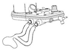
Figure 2-9 Breathing circuit connection view
