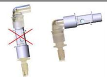
To keep secretions and moisture from pooling on the windows or oxygen sensor port, always position the IRMA probe in a vertical position with the LED pointing upwards.
