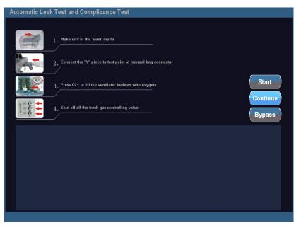
Figure 5-3 Vent mode leakage test and compliance test screen
