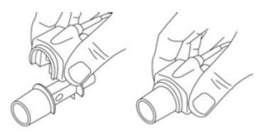
Figure 6-3 IRMA probe connection view
