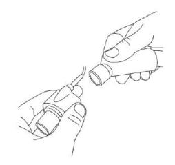
Figure 6-5 IRMA airway adapter connection view I
