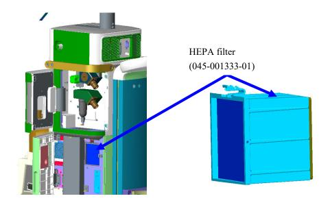
(3) Replace the air inlet dust screen (045-001298-01) every 12 months as required. Remove the HEPA filter.
