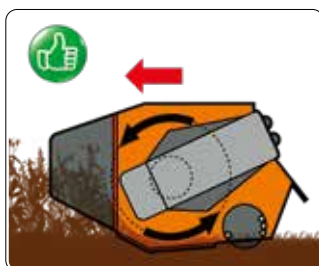
Rotore a denti fissi con riporti al tungsteno. Rotor, fixed teeth with tungsten coating and rotor with steel profiles.
