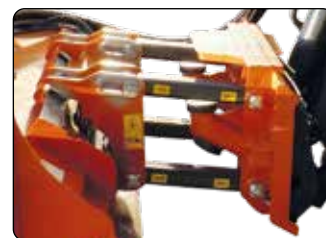
Attacco SAE J2513. Universal coupling SAE J2513.
