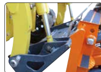
Attacco SAE J2513. Universal coupling SAE J2513.
