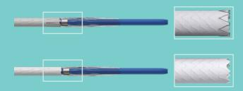
2. The connector width has been increased by approx. 20% to improve the longitudinal stiffness of the stent.
