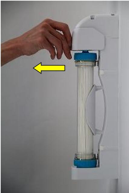
1. Pull the Swing cover to the arrowed direction.
