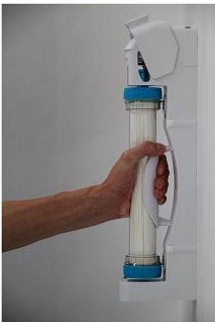
1. Insert the CF inlet and CF flushing line to each port of the CF holder, and firmly grip the CF and CF guide together.
