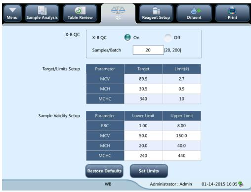
On the X-B QC setup screen, you may activate/deactivate X-B QC, set target/limits, and configure the sample validity setup.
