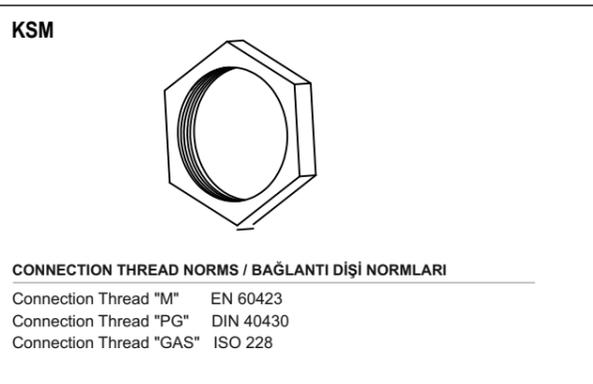
**CONNECTION THREAD NORMS / BAĞLANTI DIŞI NORMLARI**
