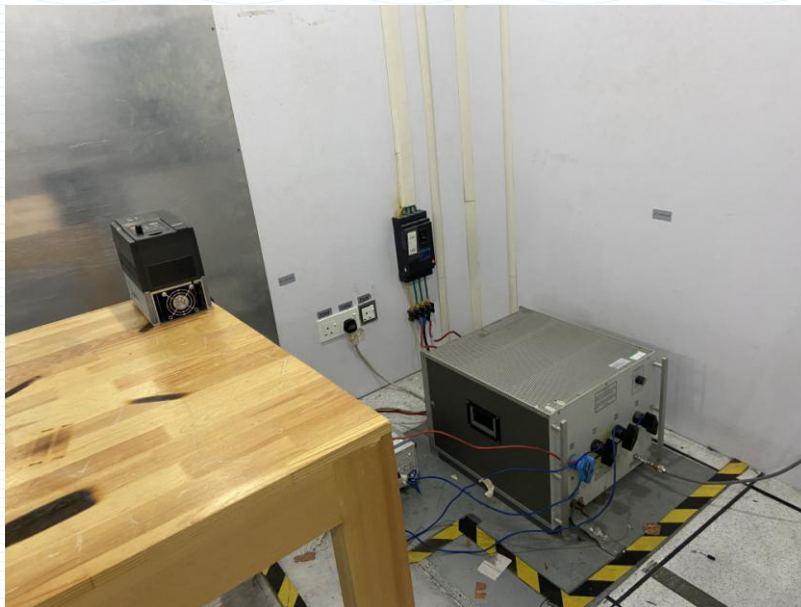
Figure 1 POWER LINE CONDUCTED TEST OF EUT
