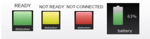
This area contains indications of the detector connection status, the battery charge level, the amount of free space (%) on the archive disk and equipment status warnings and alarms.
