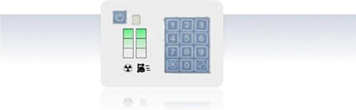
Numeric keypad for secure on/off system routine, with Four-digit access code.
