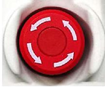
In the event of an emergency, the unit is turned OFF by forcibly pressing this switch (red mushroom-shaped switch). The switch is protected by the Cover, in order to prevent it from being accidentally pressed.
