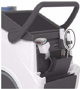
Radiographic exposures are controlled with the “Prep” (preparation) and “Exp” buttons on the X-ray Handswitch.
