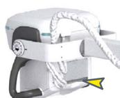
The external DAP Chamber (Radiation Meter) is installed in the lower guide of the Collimator rails. It reads the radiation as Dose Area Product (DAP) in  $\text{mGy}\cdot\text{cm}^2$  (*for further information, refer to Section 4.5 of "Dosimetry"*).
