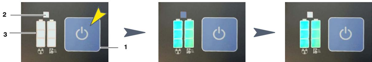
The system in the ON status switches ON the Generator, allowing the Mobile motion and then, the Image Acquisition Software for Radiographic operation will be launched on the Control Console.
