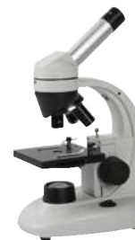
BM-44 1.Eyepieces:10X 2.Objectives:4X,10X,40X 3.Coarse Adjustment Range:8mm 4.Working Stage:90mmx90mm 5.Condenser:NA0.65 abe condenser 6.Illumination:LED light
