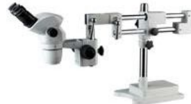
BM-500-XTWZII 1.WF10X/22mm diopter adjustment eyepiece 2.Objective:0.67x-4.5x 3.Working distance:105mm 4.XTWZII boom stand
