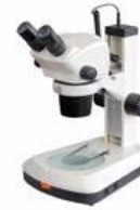
BM-217 1.Eyepiece:WF10X/23 3.Objective:Zoom range 0.63X-5X,Zoom ratio:1:8 4.Working Distance:110mm 5.Up and Down Halogen bulb 12V/15W
