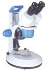
BM-205 1. 1.45° inclined, 360° rotatable binocular head 2. Wide field, high-point eyepiece WF10X 3. Objective: 2x/4x, 1x/2x and 1x/3x for option 4. Working distance: 100mm 5. L1 stand with LED illumination 6. New design with handle
