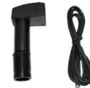
MD35 1. 1.1/4" 0.35MP color CMOS imaging module 2. 640*480 active pixels 3. Frame rate:30fps@ 640*480
