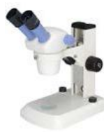
BM-N-405 1.Wide field eyepiece:10X/20mm 2.Zoom objective:1x-4.5x 3.Working Distance:97mm 4.LED illumination
