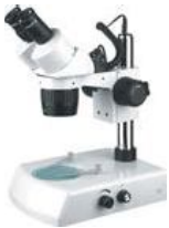
BM-204 1. 1.45° inclined, 360° rotatable binocular head 2. Wide field, high-point eyepiece WF10X 3. Objective: 2x/4x, 1x/2x and 1x/3x for option 4. Working distance: 100mm 5. B2 stand with illumination
