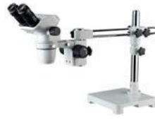
BM-500-XTWZ1 1.WF10X/22mm diopter adjustment eyepiece 2.Objective:0.67x-4.5x 3.Working distance:105mm 4.XTWZ1 boom stand
