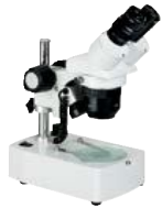
BM-SM20 1. 1.45° inclined, 360° rotatable binocular head 2. Wide field, high-point eyepiece WF10X 3. Objective: 2x/4x, 1x/2x and 1x/3x for option 4. Working distance: 80mm 5. Incident & transmitted illumination: Halogen bulb 12V/10W
