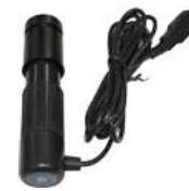
MD10 1. 1.1/7" 0.1MP color CMOS imaging module 2. 352*288 active pixels 3. Frame rate:30fps@ 352*288
