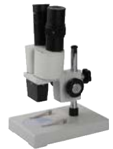
BM-XT2B 1.Eyepiece:WF10X 2.Objective:4X 3.Illumination:natura lamp 4.Coarse adjustment range:40mm 5.Working distance:70mm
