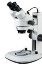
BM-400J3 1. High point WF10X/20mm 2. Objective: 0.7x-4.5x zoom 3. Working distance: 100mm 4. Reflected and transmitted LED illumination 5. Stand Size is 285x238mm
