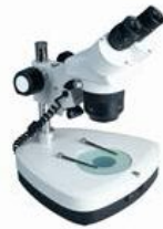
BM-SM20-C2 1. 1.45° inclined, 360° rotatable binocular head 2. Wide field, high-point eyepiece WF10X 3. Objective: 2x/4x, 1x/2x and 1x/3x for option 4. Working distance: 80mm 5. Incident & transmitted illumination: Halogen bulb 12V/10W
