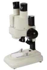
BM-20X 1.Total Magnification:20X 2.Eyepiece:WF10X 3.Objectives:2X 4.Top Light:LED Electrical Illumination
