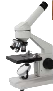
BM-41 1.Eyepieces:10X 2.Objectives:4X,10X,40X 3.Concave-Plano Reflector 4.Coarse Adjustment Range:8mm 5.Working Stage:90mmx90mm 6.Condenser:NA0.65 abe condenser
