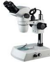
BM-500B 1.WF10X/22mm diopter adjustment eyepiece 2.Objective:0.67x-4.5x 3.Working distance:105mm 4.Reflected and transmitted,12v/15w halogen lamp
