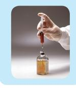
Insert Oxoid Signal growth-indicator chamber device and place system on an orbital shaker for the first 24 hours of 7-day incubation period
