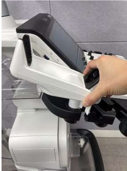
Figure 3-4. Install TVTR Probe holder
