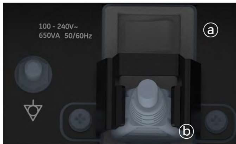
Figure 3-8. Circuit Breaker (a) and Power Plug (b)
