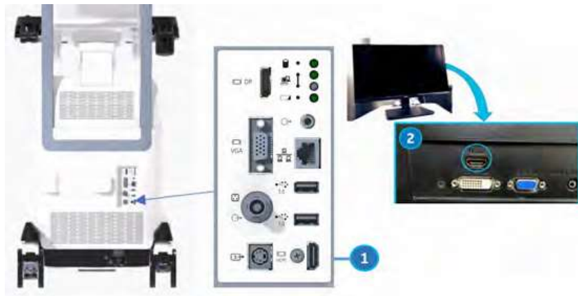
Figure 3-7. Connect HDMI Cable to back of LOGIQ Totus and External Monitor
