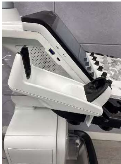
Figure 3-5. TVTR Probe Holder
