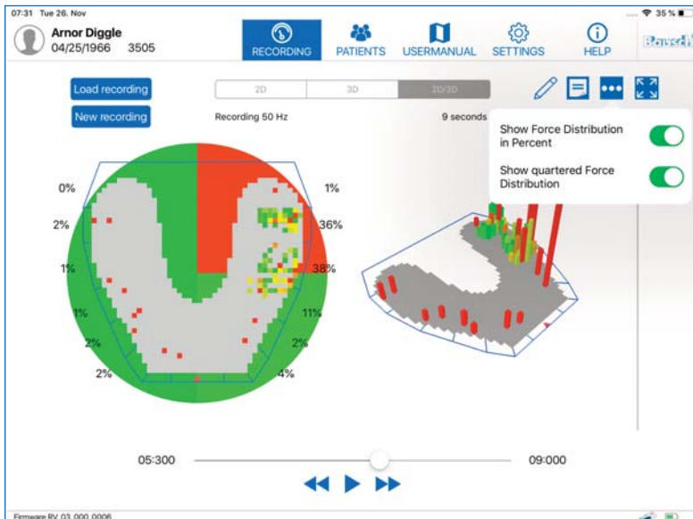
Figure 46: Occlusal pressure with both options for the occlusal force distribution enabled
