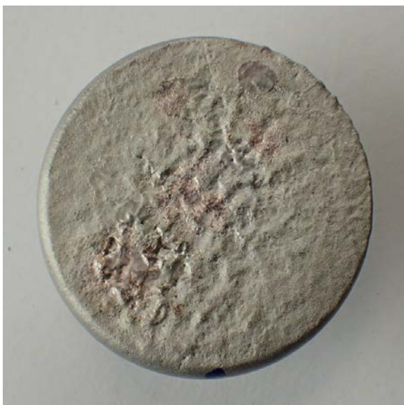
Picture 4a: Movable transition contact (TTVb).
