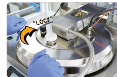
Safety lock with 12 hooks !
