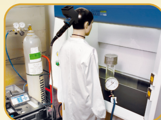
Tracer Gas (SF 6 ) Containment Test
