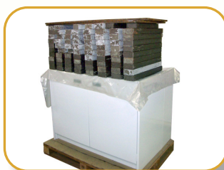
Actual photo during Cabinet Load Testing
